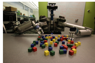
Figure 2.1: Herb (Home Exploring Robotic Butler) [Srinivasa et al., 2010] is picking up blocks from the tabletop.
