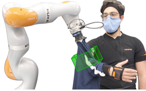
Figure 1.3: In robot-assisted dressing, parts of the human body (such as the elbow) may be occluded from sensors. This thesis introduces a state estimation algorithm that explicitly models uncertainty in both human motion and sensor observations. By representing and respecting this uncertainty, the robot produces more reliable estimates, which is critical for safe physical assistance [26].
