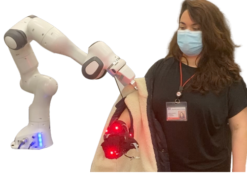
Figure 6.1: During robot-assisted dressing, the robot must remain physically close to the human arm to ensure human comfort due to the limited size of the armhole. Robot motion planners optimizing for human safety, defined as collision avoidance, might cause the robot to freeze under uncertainty, stalling progress. This chapter redefines safety to allow either collision avoidance or low-impact contact, enabling the robot to complete the task efficiently without compromising safety.
