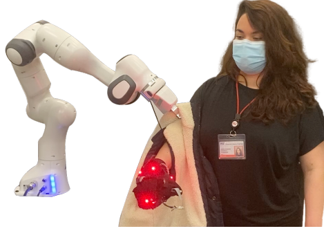
Figure 1.4: When assisting a person during dressing, the robot must plan safe motions under uncertainty about human behavior. Traditional safety constraints often prohibit any contact, leading to robot freezing [49]. This thesis proposes a relaxed safety definition that allows either collision avoidance or low-impact contact, enabling the robot to continue assisting effectively even under uncertainty [25].
